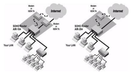
Figure 1-1 Internet Access with the AIR-104/204
